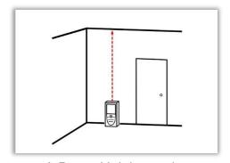
A Room Height can be measured anytime during measuring process
